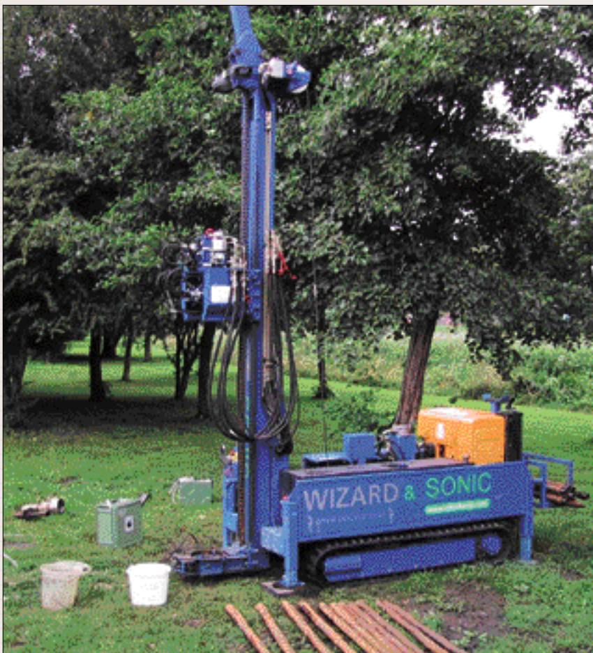
Wizard drilling rig with Sonic drill module
