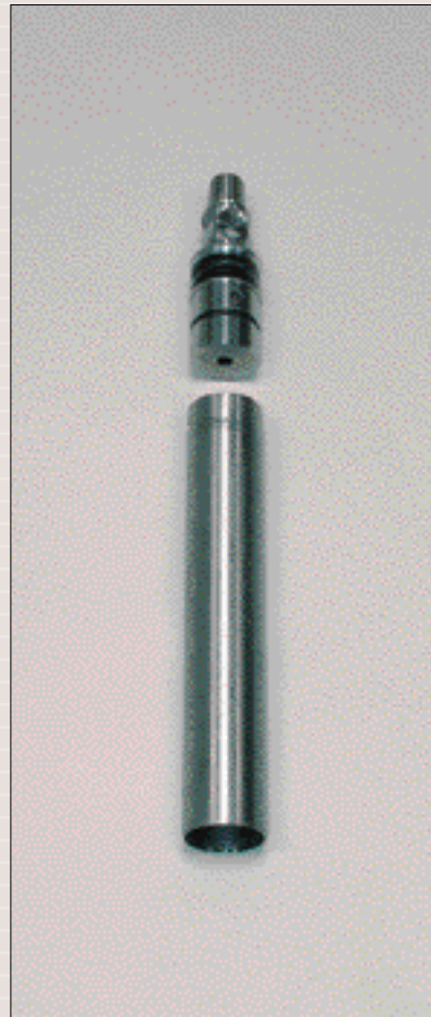
Coring apparatus with sample tube
