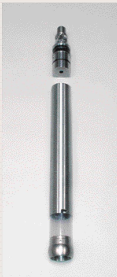
Coring apparatus, tube, cutting head
