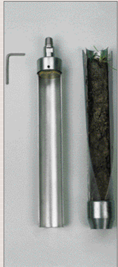
Split tube sampler with sample in liner
