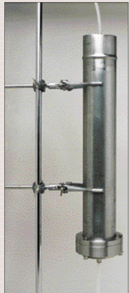
Connection set for leaching tests
