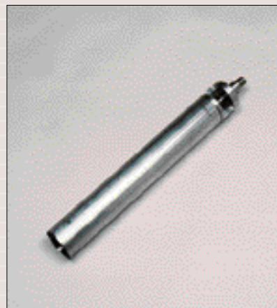
Van der Horst core sampler with tube
