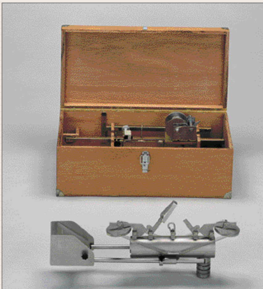
Water sampler 'Watertrap', complete set
