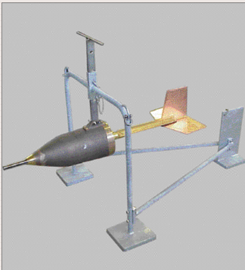
Suspended load sampler Delft bottle type
