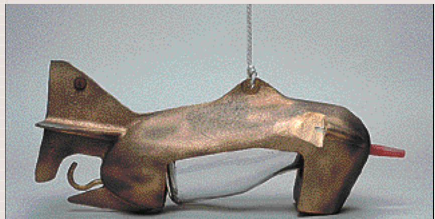
Sampler for suspended sediment
