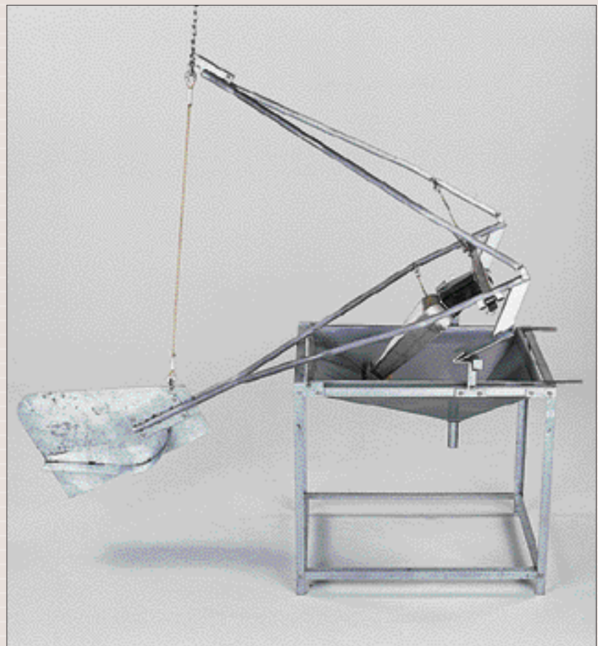
Bed-load transport meter, Arnhem type
