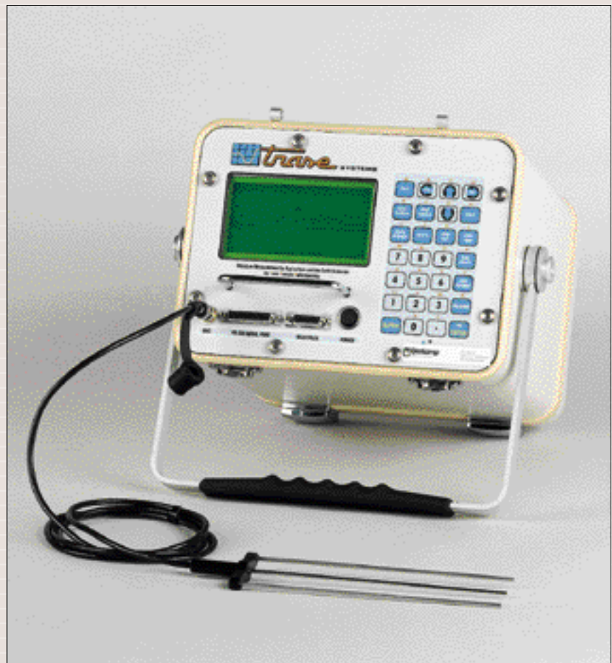
Trase soil moisture measuring system
