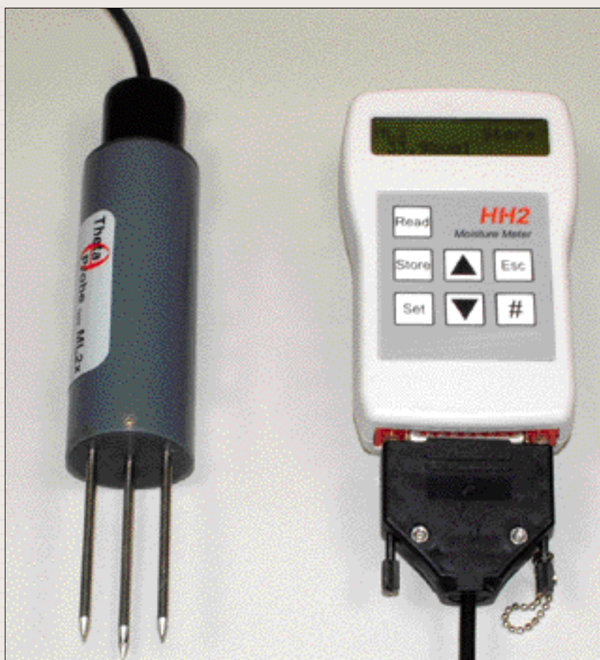
Soil moisture meter with soil moisture sensor Thetaprobe
