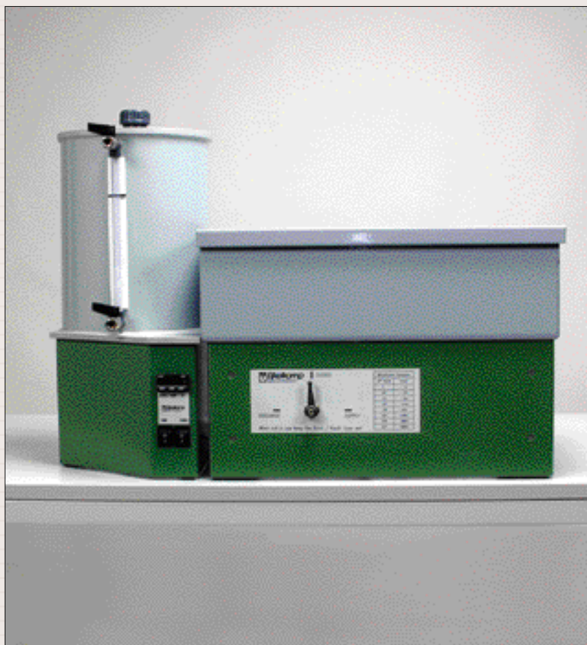
Sand/kaolinbox for pF-determination (pF 2.0 - 2.7)
