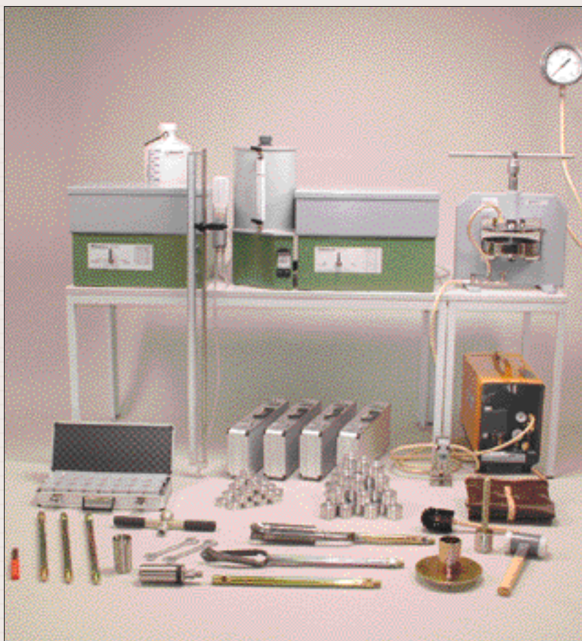
Set for pF determination, sandbox method (pF 0 - 4.2)
