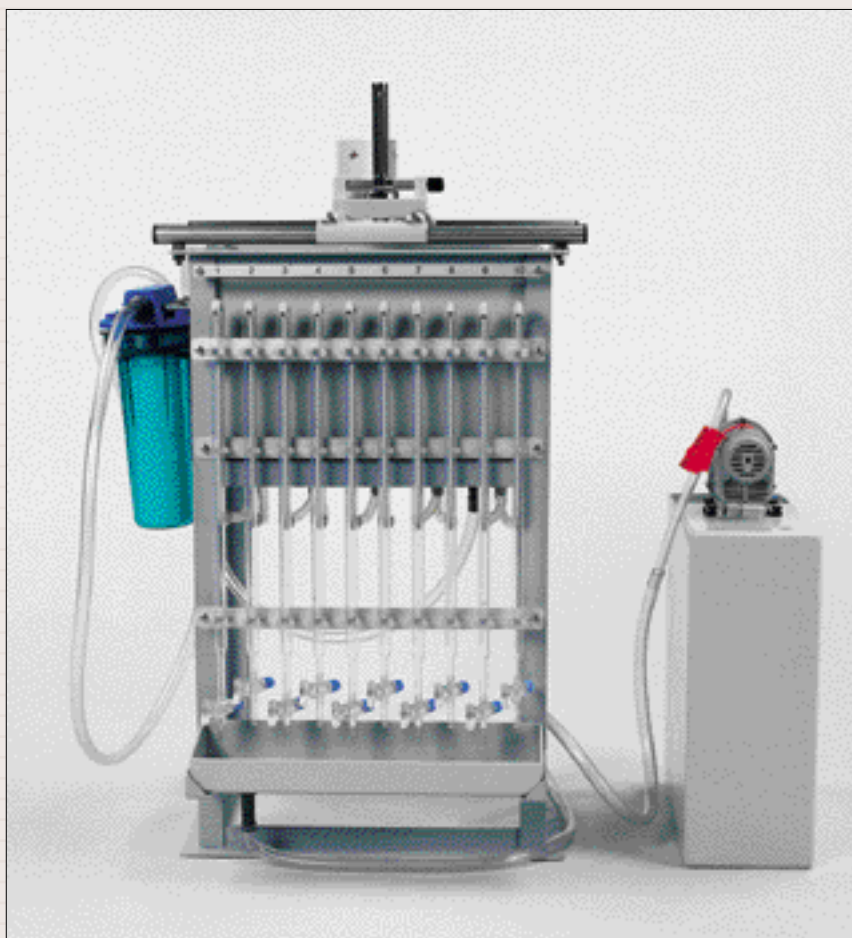
Soil water permeameter for 10 samples, closed system
