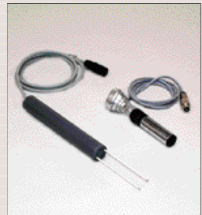
Tensiometer and soil moisture sensor
