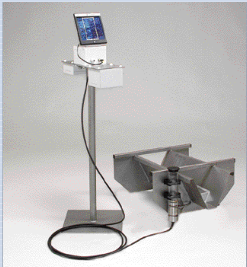
Small RBC flume with pressure transducer, logger and solar panel
