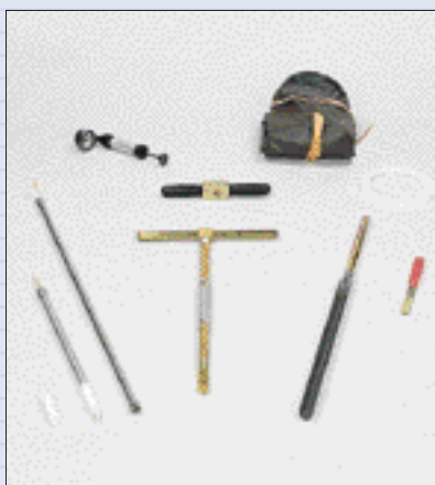
Soil moisture sampling system (SA)
