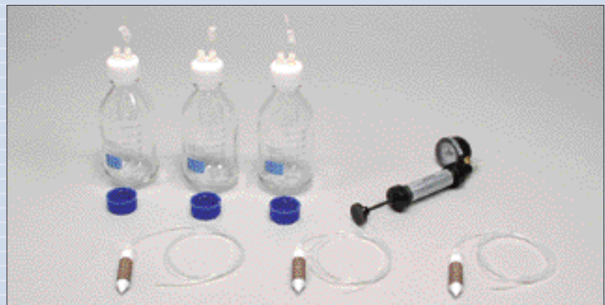
Soil moisture sampling system with teflon/quartz probes
