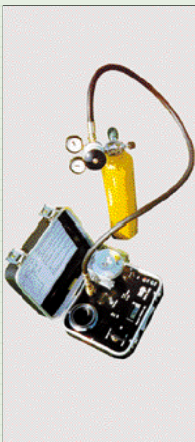
Digital plant moisture system
