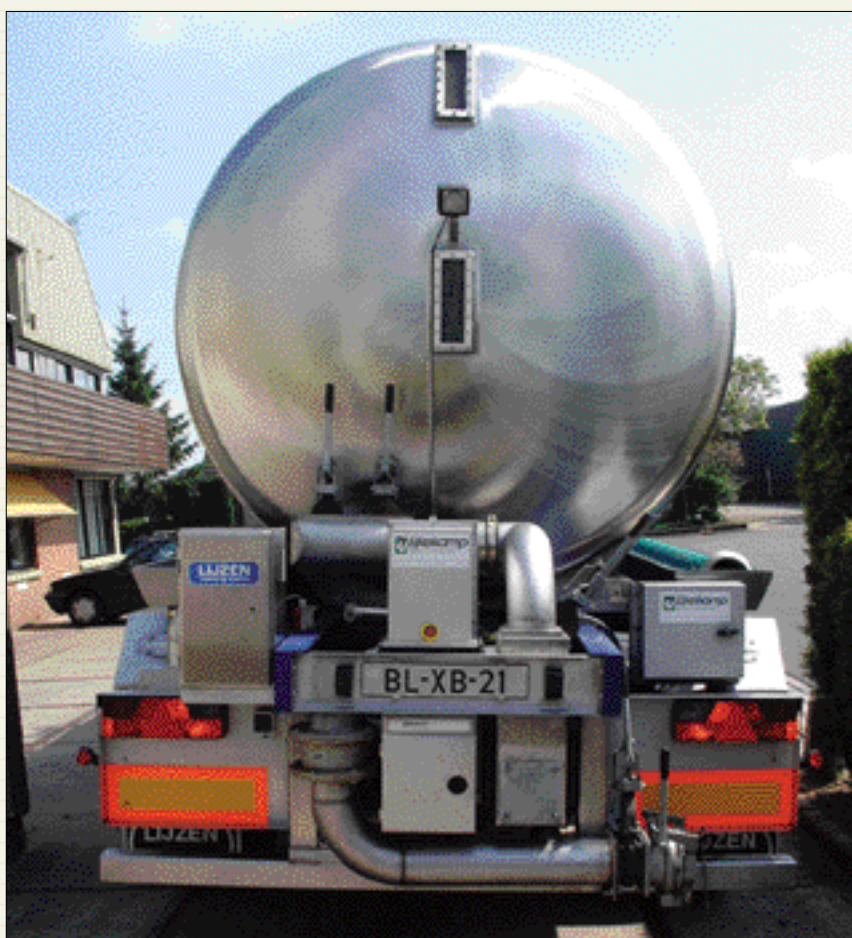
Automatic fraud-proof sampling system built on a tank lorry
