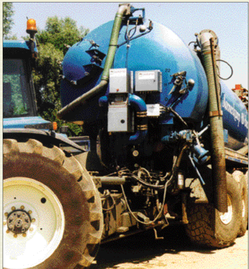
Automatic sampling system built on a tank pulled by a tractor
