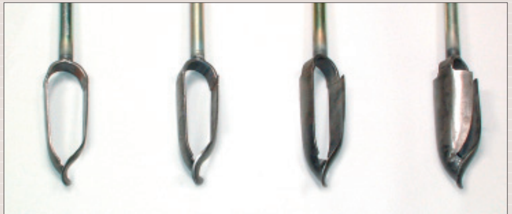
Edelman augers: clay, combination, sand and coarse sand type
