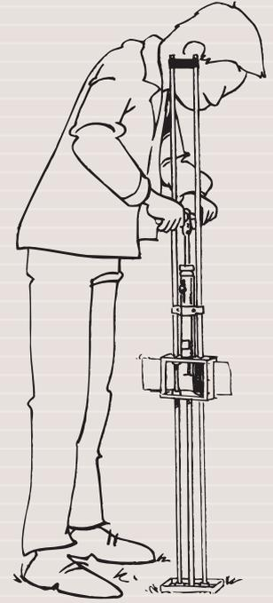
The cone check is used to inspect the wear of the cones.
