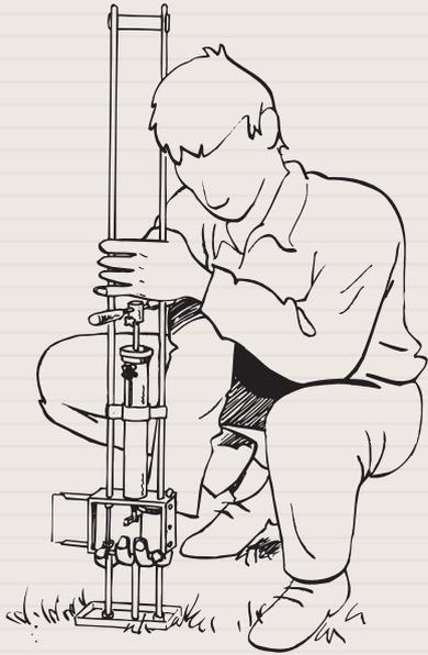
In addition, the penetrometer is self-recording, i.e. during the measurement the resistance is immediately graphically recorded. This greatly reduces the amount of work to be done afterwards, the data can be immediately transferred and it is easy to store.
