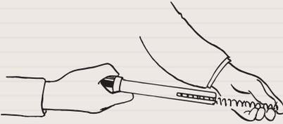
At this point the spring takes a slip ring along. This slip ring indicates on the scale the maximum compression measured up to that time.
