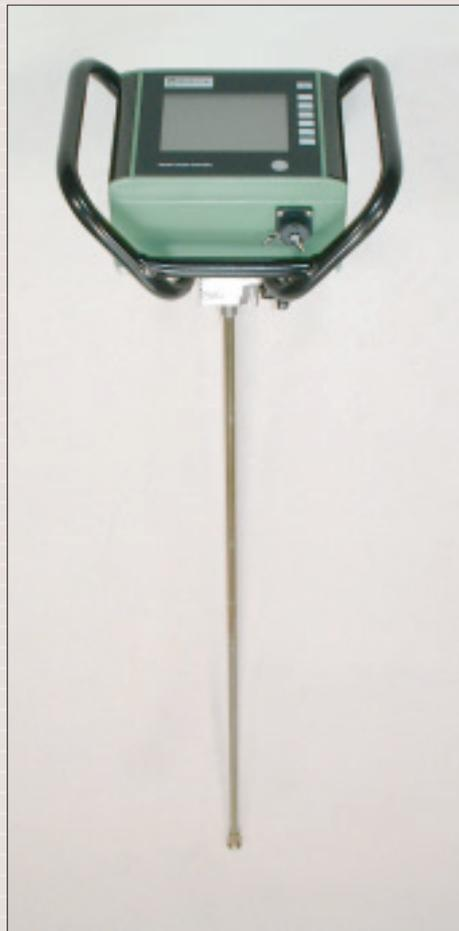
Penetrologger, probing rod and cone
