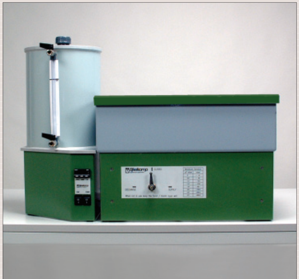
Sand/kaolinbox for pF-determination (pF 2.0 - 2.7)
