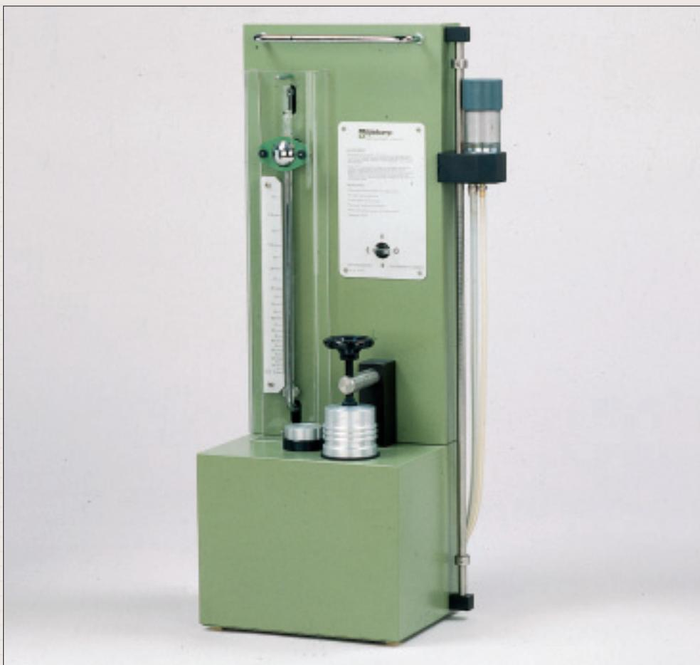
Air pycnometer according to Langer
