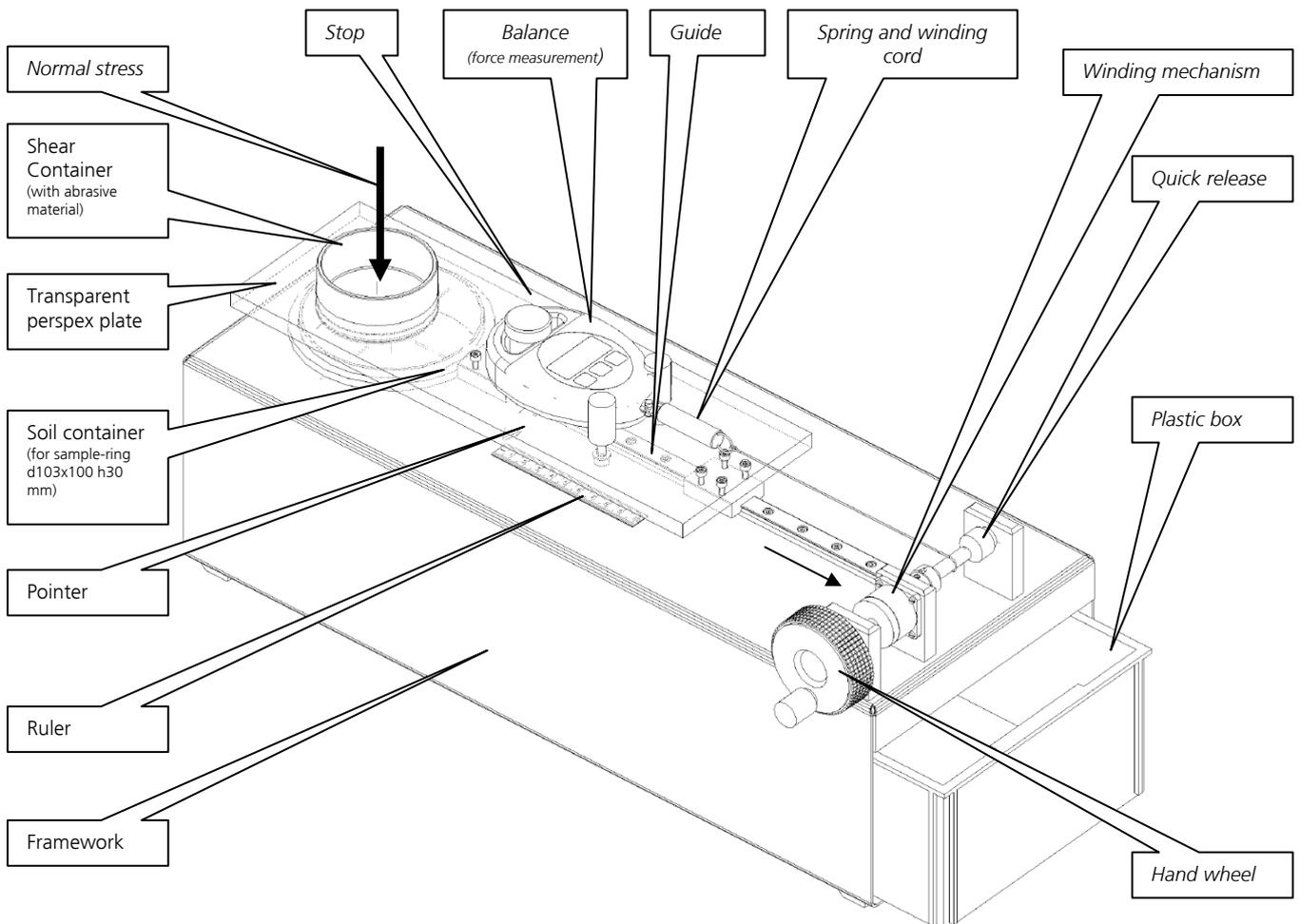
*Schematic representation of surface shear apparatus*
