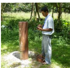
Groundwater Monitoring site Data readout via HDA
