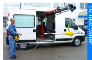
vehicle with crane and current meter
