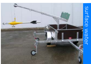
SEWII with mobile jib and current meter
