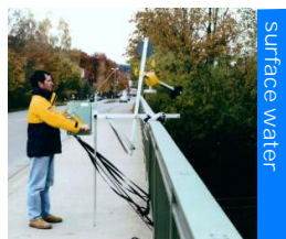
mobile bridge jib
