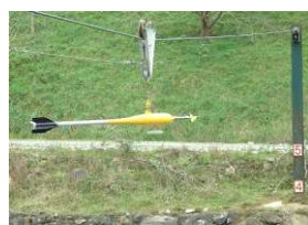
Universal current meter in use
