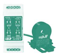
The Ampere / mA converter is used for monitoring of motor current where the motor current from one of the phase conductors is converted to a mA signal, so the motor current can be used for control, monitoring and recording.
