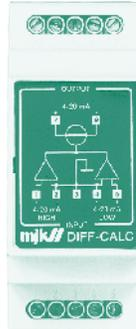
Diff-Calc transmits a 4-20 mA signal proportional to the difference between two 4 - 20 mA signals from transmitters. Diff-Calc is especially designed for measurement of level differences where Diff-Calc is connected to two ultrasonic or pressure based level transmitters. Diff-Calc can be used with any 4 - 20 mA signals, such as temperature differential or the difference between pH values, etc.
