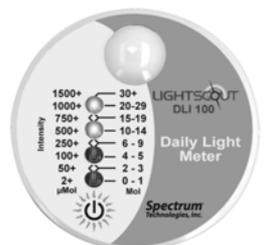
During the Light Gathering period, by reading the **left** numbers, the light intensity would be in the range 750-999  $\mu\text{mol}\cdot\text{m}^{-2}\cdot\text{s}^{-1}$  (“750” is between the two lit LEDs, and the top of the range is less than 1000, the next number up).
