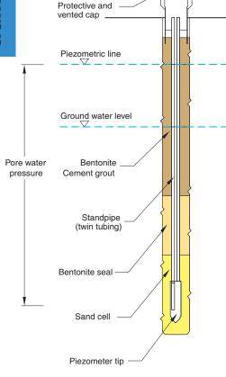
Casagrande piezometers are used to detect, measure and monitor water pressure in permeable soil or rock specifically at the installed depth of the measuring tip. Typically a bentonite seal is installed immediately above and sometimes below the filter. The filter is normally connected to the surface by a pair of tube columns.
