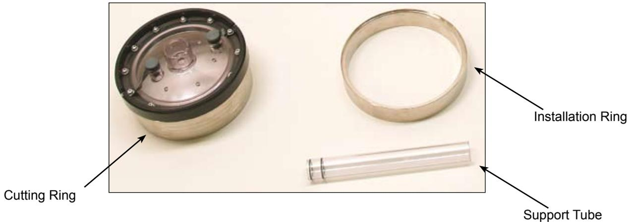
Figure 2 - Pressure Infiltrometer Foot Assembly, Disassembled
