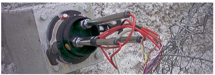
MPBX head with displacement transducers, installed on retaining wall
