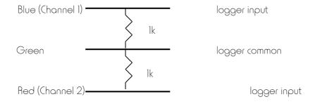
If a precision resistor of IK (0.1% ppm/deg.C.)\* is used, then the output in mV of the sensor will be identical to the current output in  $\mu$ A. For example, if the calibration certificate says Channel 1 output is 30.25  $^{2}\mu$ mol m<sup>-2</sup> s<sup>-1</sup> per  $\mu$ A, then when connected with a  $1k\Omega$  resistor, 30.25  $^{2}\mu$ mol m<sup>-2</sup> s<sup>-1</sup> will give an output of 1mV.
