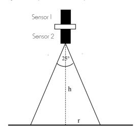
Sensor 1 is cosine corrected and is measuring incident light.
