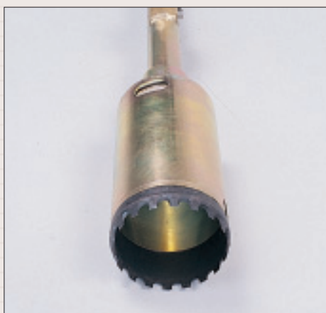
Drilling-crown, extruder in upper position
