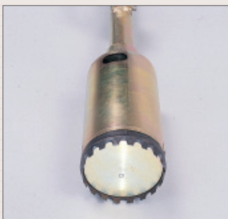
Drilling-crown, extruder in lower position
