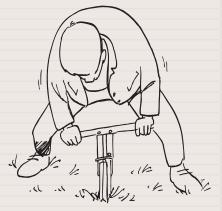
Once the required depth has been reached, the profile sampler is extracted from the soil in a clamped position.
