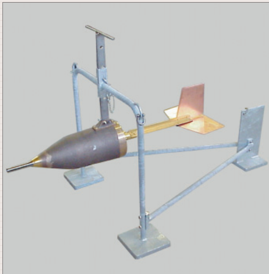
Suspended load sampler Delft bottle type
