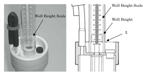
Fig. 27. Connecting the Well Head Scale to the Reservoir Cap
