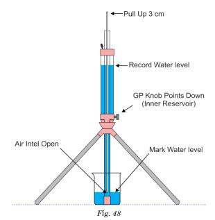
**Check the water level** in the Inner Reservoir after approximately one hour. If the system is not leaking, the water level in the inner Reservoir should be the same as recorded previously. Also the water level in the Beaker should not rise.
