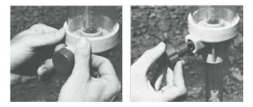
Fig. 37. Removing Reservoir Valve.
