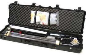
Fig. 2 Guelph Permeameter Carrying Case.
