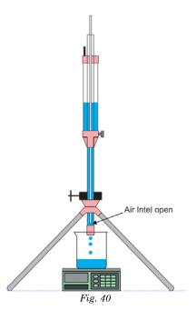
**Push down the Air Tube** to seal the Water Outlet Tip when the water level in the Reservoir is close to the bottom (water level about 70 cm). This should stop water flow out of the Water Outlet Tip and also the falling water level in the Reservoir.
