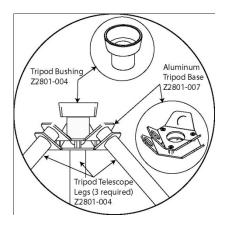
Fig. 10. Tripod Assembly
