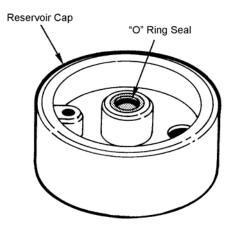
Fig. 14. Illustration of Reservoir Cap and O-Ring position.
