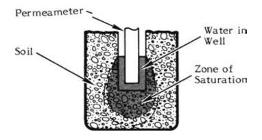
Fig. 4. Saturated zone around borehole (saturation bulb).
