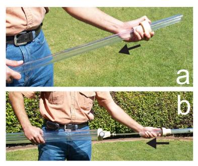
Fig. 23. Assembling the Tripod Bushing and Support Tube.
