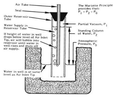
Fig. 3. In-hole constant-head permeameter setup
