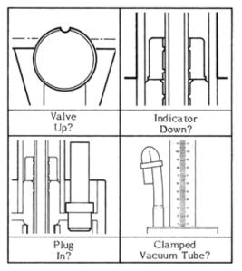
Fig. 30. Double check these items before each reading
