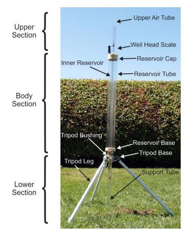
Fig. 7. Guelph Permeameter main components.
