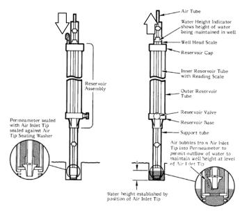
Fig. 12. Illustration of Air Inlet status. Left: closed/sealed state (push the Air Inlet Tube all-the-way down). Right: open/operating state (pull the Air Inlet Tube to the desired water head height).
