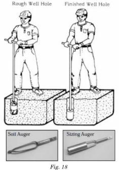
The Sizing Auger, shown in Fig. 18, is used as a finishing tool to produce a proper sized well hole uniform geometry, meeting the size and shape requirements of the model, and to clean debris off the bottom of the well hole. The Sizing Auger is designed to produce a hole that is uniformly 5 cm in diameter with a flat bottom. It is also important to keep the blade sharpened to a knife-blade edge in order to minimize smearing.
