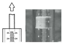
Fig. 33. Raise the Air Inlet Tip by slowly pulling up the Upper Air Tube.
