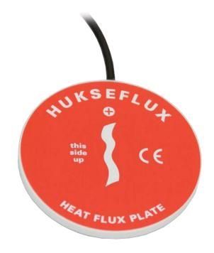
The HFP01 is for applications that do not require self calibration.
