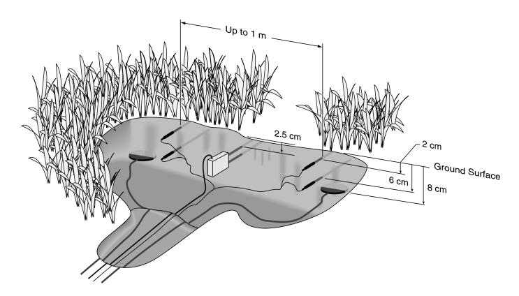
The above illustration shows heat flux sensors installed with the CS616 and TCAV Averaging Soil Temperature Probes. All sensors must be completely inserted into the soil face before the hole is backfilled.
