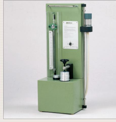
Air pycnometer according to Langer
