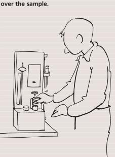
As soon as the under pressure is stable the value can be read and the levelling vessel is placed in the upper position.
