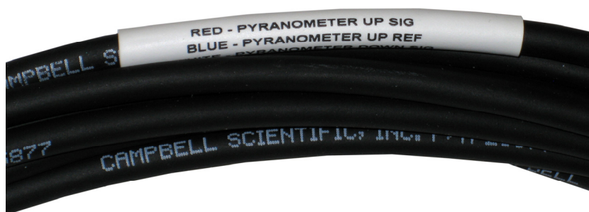
FIGURE 6-3. Labels on the pigtail end of the SOLAR cable.
