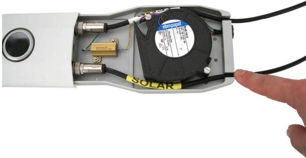
FIGURE B-3. Making sure the cables are clear from the edges.
