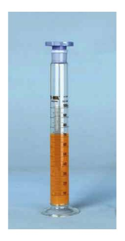
With interchangeable polyethylene stopper and glass foot.
