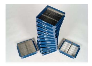
A range of 14 different grid sieves are available from Impact. The frames are painted steel with stainless steel bars. Nominal dimensions: 300mm x 300mm x 75mm high.
