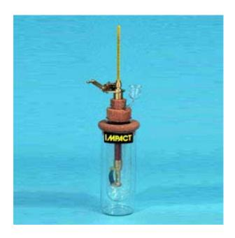
This apparatus is used to determine the breaking point of semisolid and solid bitumens.
