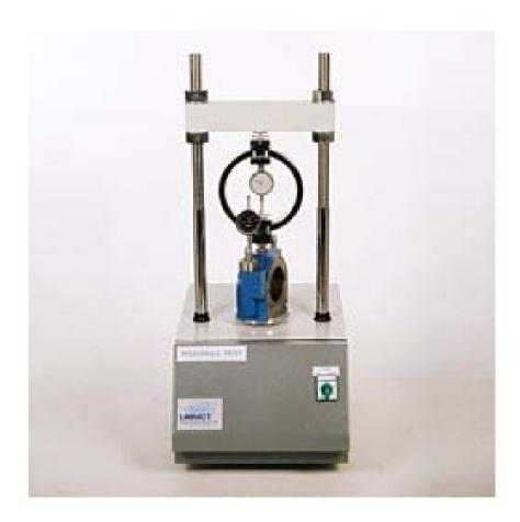
The Impact BM220 Marshall machine is a motorised load frame specifically designed to carry out Marshall tests.
