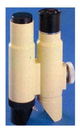
Portable microscope for measuring cracks in concrete and other materials.
