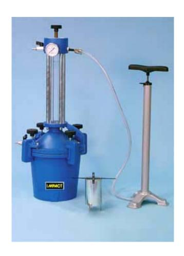
Made from cast aluminium alloy, this type A air entrainment meter records the percentage of air entrained in freshly mixed concrete.
