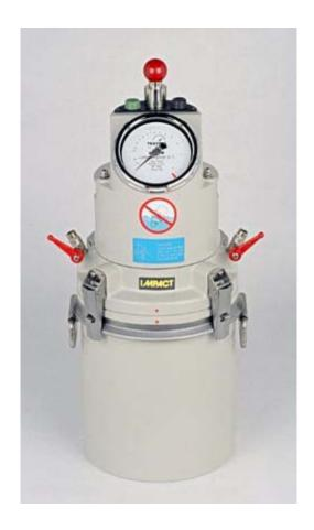
Air entrainment meter for freshly mixed concrete, with manually operated pump.
