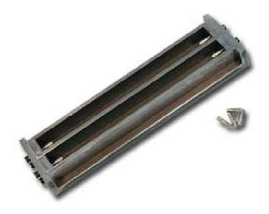
Two gang prism mould to produce 25mm x 25mm x 250mm sample for expansion tests in an autoclave.
