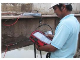
\* Readings are stored in an internal SD card and the stored data can be fast and easily transmitted to a host PC by USB cable.
