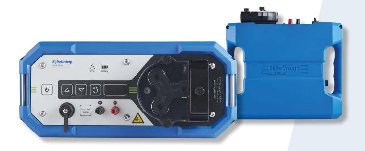
This peristaltic pump suitable for field use (item no.: 1235) is battery-powered and is microprocessor controlled. The microprocessor provides adjustable constant speed, overload protection and various external control functions. A built-in maintenance-free 12 Volt lithium-ion battery (10 Ah) makes it possible to use the pump for two to five hours at a time (depending on the load). The housing is the highest degree splash-proof (IP 66) and can function safely and without problems in the field.
