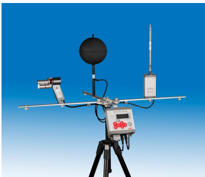
R-Log (ELR510.1) tripod mounting using a stand.
