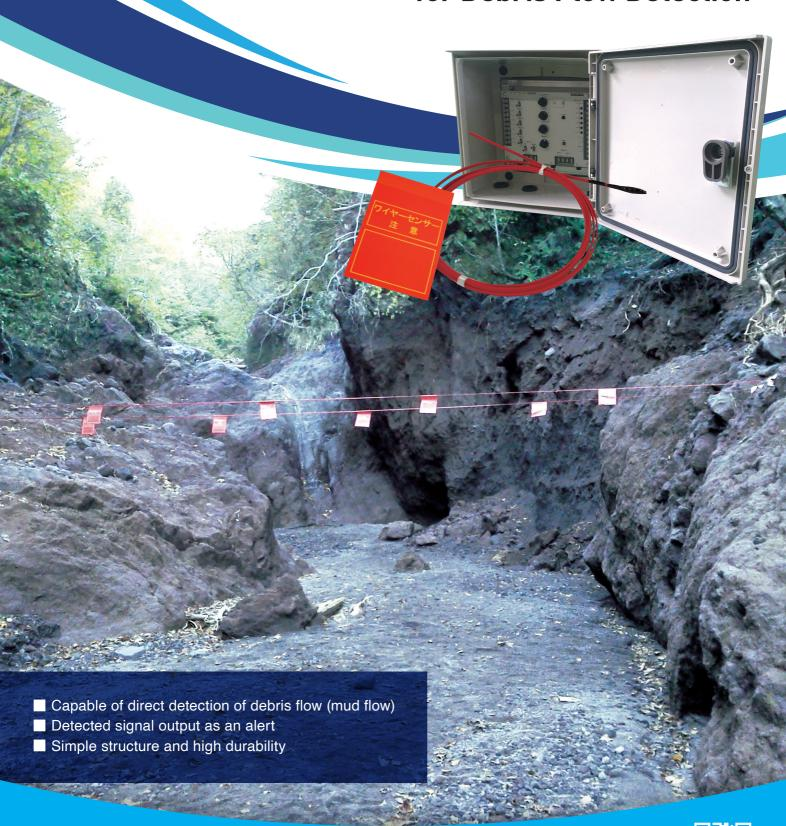
This sensor detects the occurrence of a debris flow, using a wire stretched across a mountain stream, when the debris flow (mud flow) passes through and cuts the wire. By stretching multiple wires (maximum 5 survey lines) vertically, the scope can be estimated.
